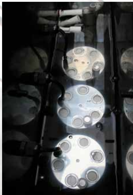
a look on the inside of the humidifier here we produce mist through ultrasonic diaphragm
